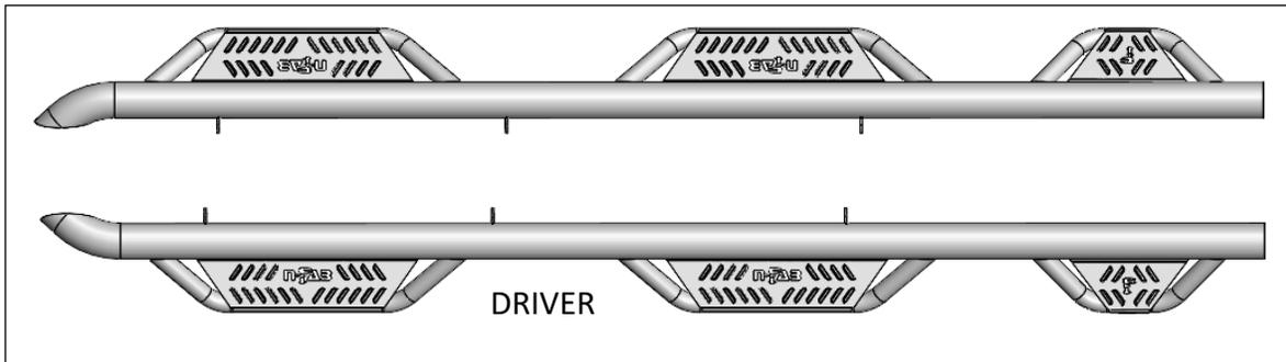
**Step 2:** Install the (x6) mounting brackets to each attachment point on the main tube using the supplied M10x25 carriage bolts, M10 hex nuts and leave loose for now.
