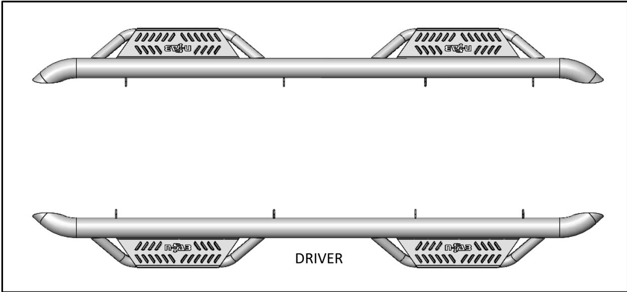
**Step 2:** Install the (x8) mounting brackets to each attachment point on the main tube using the supplied M10x25 carriage bolts, M10 hex nuts and leave loose for now.
