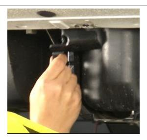
**Step 12:** Carefully place passenger side step into place. Use bolt, washer and begin hand tighten both upper mounts and pinch weld mounts to the rear two brackets. An assistant is recommended with this step.
