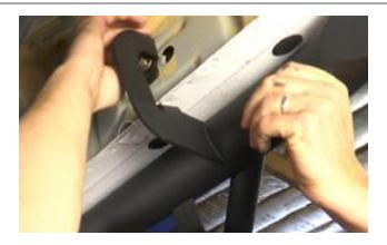
**Step 17:** Tighten all (x8) brackets at the main tube.
