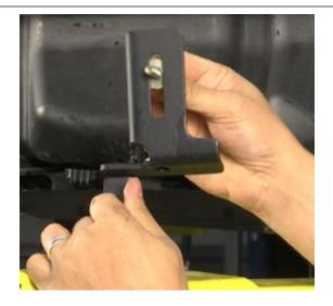
**Step 11:** Feed the bracket between the body and the DEF tank from the back of the tank. You will be able to fit, and hand tighten bolt through the bracket to the body.
