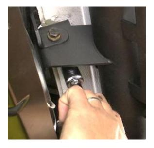
**Step 15:** Snug hardware for the first and second bracket. Tighten the bolt going up through the pinch weld first to pull the board into place, then tighten both side bolts.
