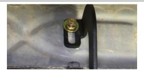
Step 5: Insert black coated bolt and washer through pinch weld hole and secure with locking nut and washer.
