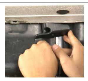
**Step 10:** The second bracket attaches to the body with a bolt rather than the tab like the first bracket.
