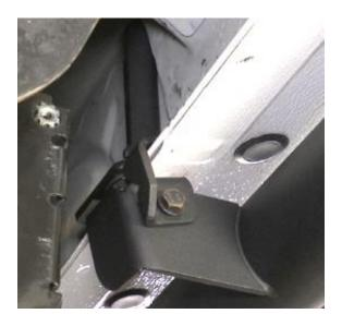
**Step 14:** Insert bolt and washer going up through step, pinch weld and through the 2 piece bracket.
