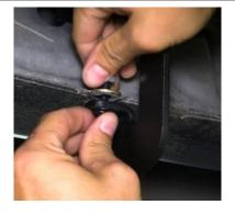
**Step 6:** Tighten pinch weld mounts first, then upper bolts. Tighten to 20 (ft./lbs) torque to secure the seps to the vehicle.
