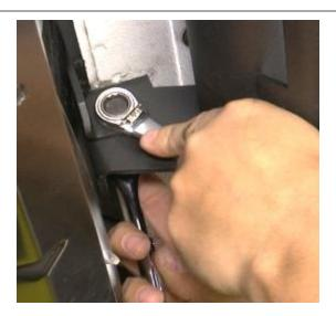
**Step 16:** Tighten pinch weld mounts first then upper mounts. Tighten all hardware to 20 (ft./lbs.) torque to secure to vehicle.
