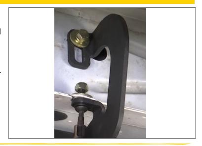
Step 12. Use (#9) M8 hex bolt, (#10) flat washer and (#11) lock nut to fasten the step to the bottom portion of (#5) and (#6) brackets.
