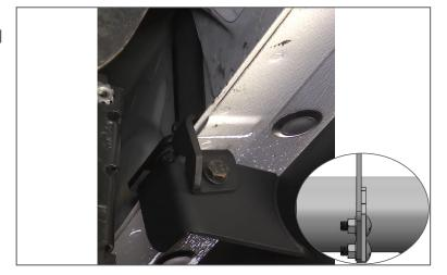
Step 16. Re-install the def tank cover.
