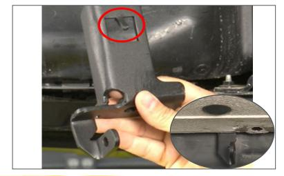
Step 8. Next, install (#6) second bracket using the suppled (#9) M8 hex bolt, (#10) M8 washer and (#13) M8 lock washer and leave loose for now.
