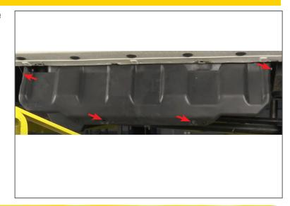
Step 7. Install (#5) first bracket by sliding up and behind the def tank until the upper tab locks into place in the body of the vehicle. Tug down firmly on the bracket until it hangs on its own and the welded nut it aligned with the hole in the pinch weld. This step may take a couple of tries.
