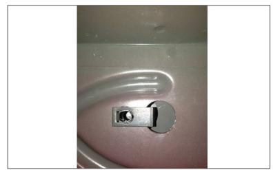
Step 3. Carefully place (#1) driver side step into place, aligning brackets with (x3) mounting locations. Use (x3)(#6) M8x35mm hex bolt, (x3)(#7) M8 flat washer and (x3)(#10) lock washer for upper mounts and leave loose.
