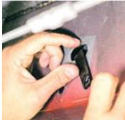
**Step 4.** Place clear retainer over stud and bolt plate. Fish bolt plate through the body of the vehicle and slide retainer tight to stud. Take your time here to avoid dropping bolt plate in the body.
