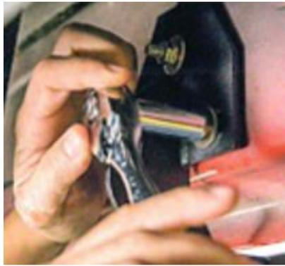
**Step 7.** After final adjustment, tighten all three brackets at the main tube.
