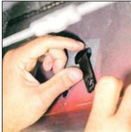
**Step 5.** Place clear retainer over stud on bolt plate. Fish bolt plate through the body of the truck. Slide retainer tight to stud. Take your time here; avoid dropping bolt plate into the body.
