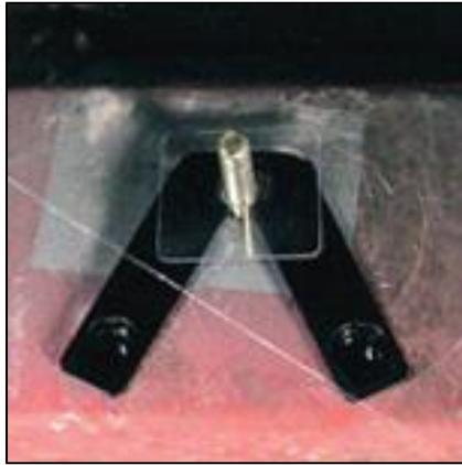
**Step 6.** Carefully place step into place. Hand tighten the upper nut to bolt plate with washer. Best to have an assistant to lift and hold step in place. Insert and hand tighten lower bolts.
