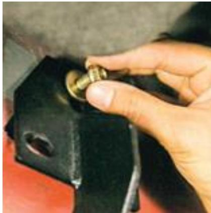
**Step 7.** Begin tightening nuts and bolts in an alternating pattern. ***Avoid using power or air tools.*** Tighten to (20 ft/lbs) torque to secure steps to truck.
