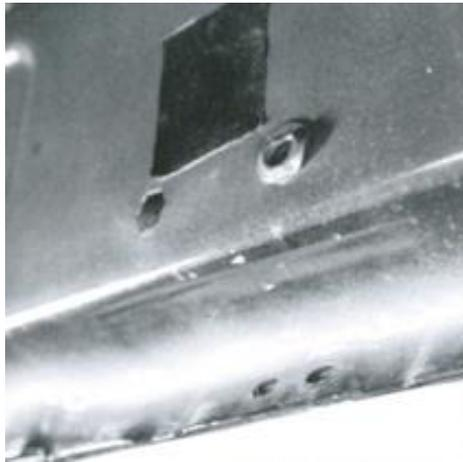
**Step 4.** Carefully place step into place. Begin with center bracket and hand tighten the upper bolt and washer to hold in place. **NOTE: An assistant is recommended for this step.** Next, insert and hand tighten front and rear upper bolts and washer.
