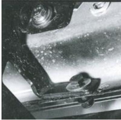
**Step 6.** Begin tightening nuts and bolts in a alternating pattern. **Avoid using power tools.** Tighten to 20 ft./lbs. torque and secure the step to the truck.
