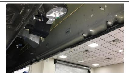
**<u>Step 3</u>**: On the inside rocker panel there will be three-attachment point consisting of three 8mm studs coming out from the panel. These studs may be covered in paint and will need to be cleaned before the installation.
