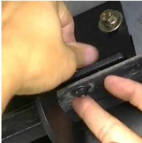
**Step 6:** *Avoid using power and air tools.* Tighten upper mounts first then pinch weld bolts. Tighten to 20ft/lb torque to secure step to the vehicle.
