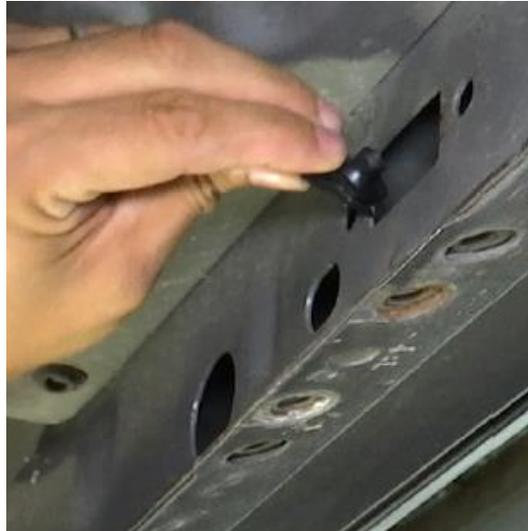
**Step 4:** Carefully place the step into the mounting position. Use the supplied M8 hex bolt and zinc flat washer and begin hand tightening (x3) upper mounts. **An assistant is recommended in this step.**
