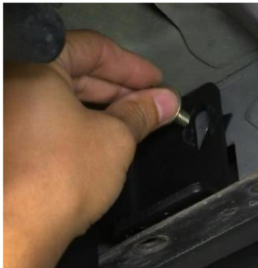
**Step 5:** Insert black button head bolt and washer through pinch weld hole. Secure with locking nut and washer.
