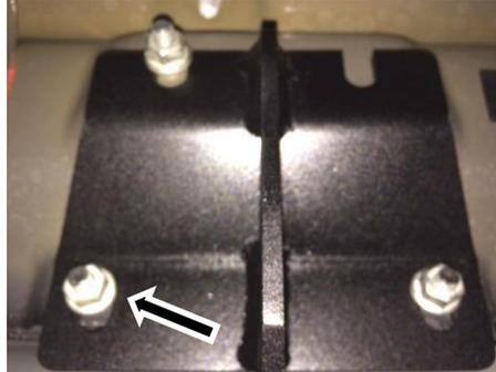
**Step 8.** After final adjustment, tighten all four brackets at the main tube.
