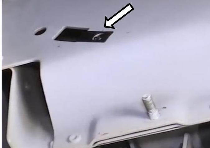
**Step 5.** Carefully raise step into position and align the three brackets with the threaded studs.
