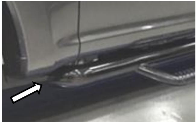
**Step 6.** Starting with the rear bracket, push up towards the pinch weld so the 3" main tube is high and tight to the body of the vehicle and use the supplied M8 nut, m8 hex bolt and washers to secure the bottom stud first.
