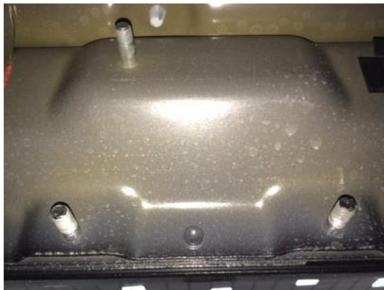
**Step 4.** Install the supplied 8mm u-nut clip in the upper body at the rear mounting location.
