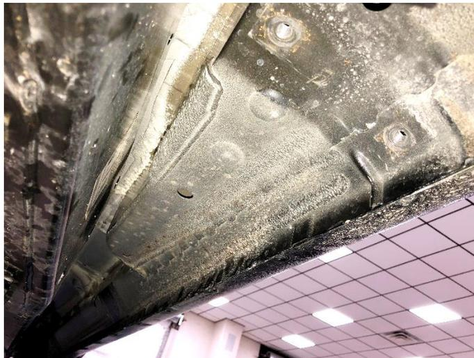
**STEP 5:** Carefully place step into place and loosely fasten using the supplied M10X25mm hardware.
