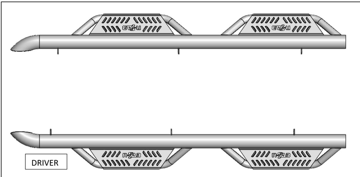
**Step 2.** Install the (x6) mounting brackets to each attachment point on the main tube and leave loose for now.
