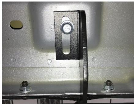
**Step 9:** After final adjustment, tighten all three brackets at the main tube.
