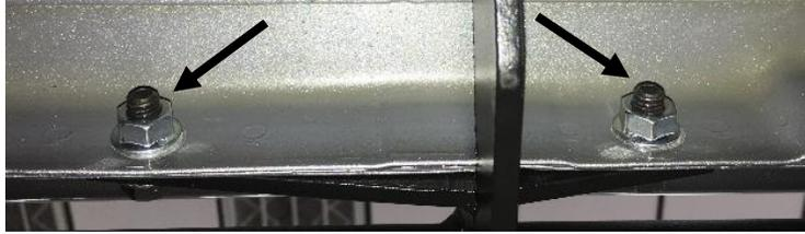
**Step 7.** First, tighten all the hardware that attaches the bracket to the pinch weld of the vehicle.
