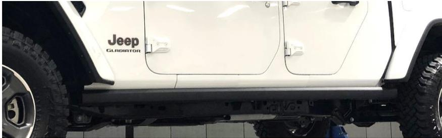
**Step 4.** Carefully raise step up into position and align the brackets with the factory mounting points with the horizontal part of the bracket on the outside of the pinch weld.
