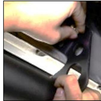
**Step 5:** Begin tighten bolts in alternating pattern. *Avoid using power or air tools.* Over tightening could strip or break the OE threaded inserts.
