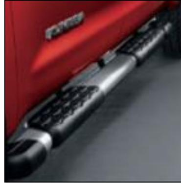
**Step 4:** Carefully place step into place. Hand tighten the upper center bolt with washers to hold in place. Next, start remaining hardware and hand tighten for now.
