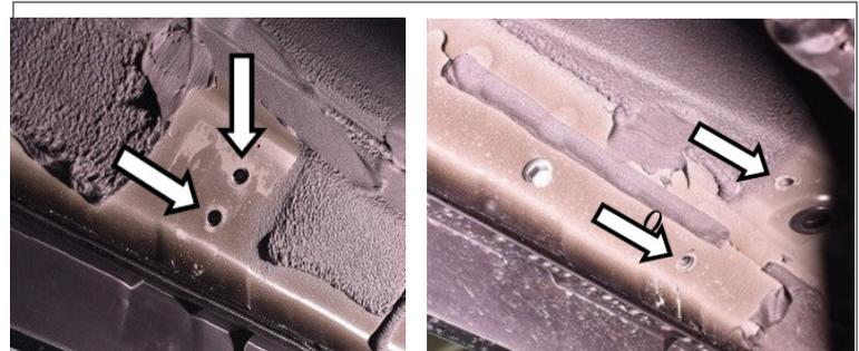
**Step 3.** Carefully place step into place aligning brackets with (x3) mounting location.
