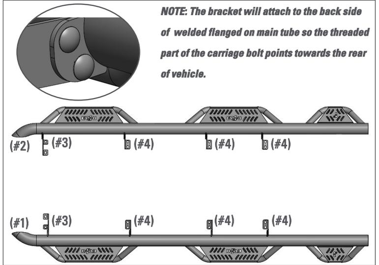
**Step 2.** Remove any OE running boards/steps and or hardware from (x3) mounting locations. Clean any dirt or debris from threaded holes.
