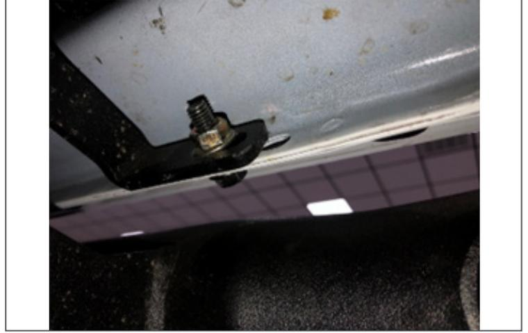
**Step 7.** Finish by tightening upper mounts. If M10x30mm bolts where used, torque to (30 ft/lbs) and (20-25 ft/lbs) for M8x30mm bolts.
