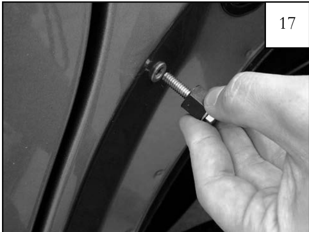
Remove rivnut tool. Repeat for remaining holes.
