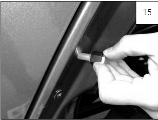
Insert rivnut in fender hole.
