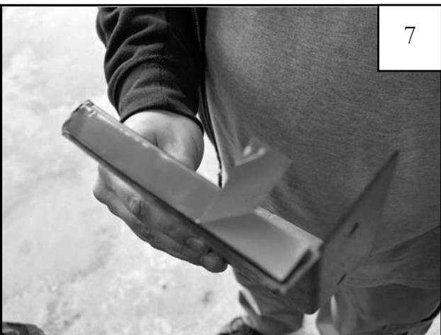
Remove the red tape liner from the Upper Protective Case for the rear wiring harness. NOTE: the tape should be facing the rear of the vehicle.
