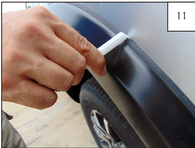
Using supplied Edge Trim Tool (ET1-0002), seat edge trim against vehicle by hooking curved end under edge trim at one end of flare. Next, slide around outer edge of flare to the other end.
