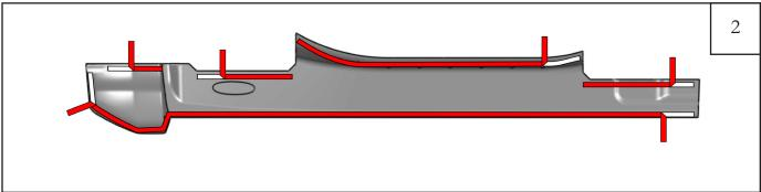
Open vehicle doors. Clean all dirt and debris from vehicle door sills and rocker panel. Use supplied alcohol wipes where part will attach.
