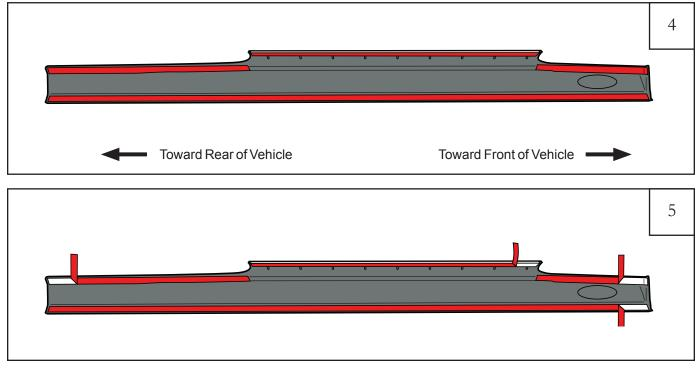
Peel back roughly 3" of red tape liner from the pieces of tape on the back side of rear part. Make sure red tape liner will be accessible when part is attached to truck. Tape layout may be different on Crew Cab part.
