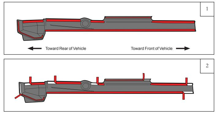
Open vehicle doors. Clean all dirt and debris from vehicle door sills and rocker panel. Use supplied alcohol wipes where part will attach.
