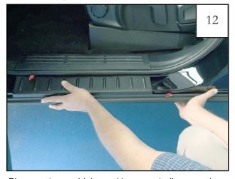
Place part on vehicle, making sure to line up edges of part with edges of vehicle. Ensure that all tape tabs are accessible. Firmly press on exposed areas of tape to tack Trail Armor in place. NOTE: Refer to step 1 for placement of certain tabs.
