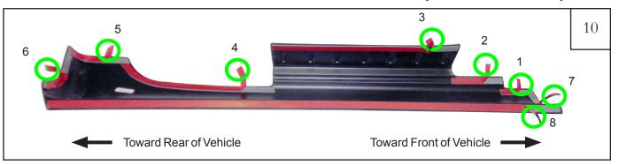
Peel back 2" of tape liner from each flange. Using a marker, number the tape tabs as shown:
