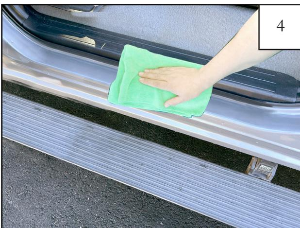
Clean all dirt and debris from vehicle then use supplied alcohol wipe where Trail Armor will be installed. *NOTE: Temperature should be at least 60°F for proper tape adhesion.*
