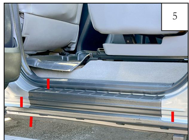
Place part on vehicle, making sure to line up edges of part with edges of vehicle. Ensure that all tape tabs are accessible. Firmly press on exposed areas of tape to tack Trail Armor in place.
