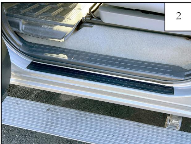
Open the rear drivers side door and locate the factory installed stick-on step plate .
