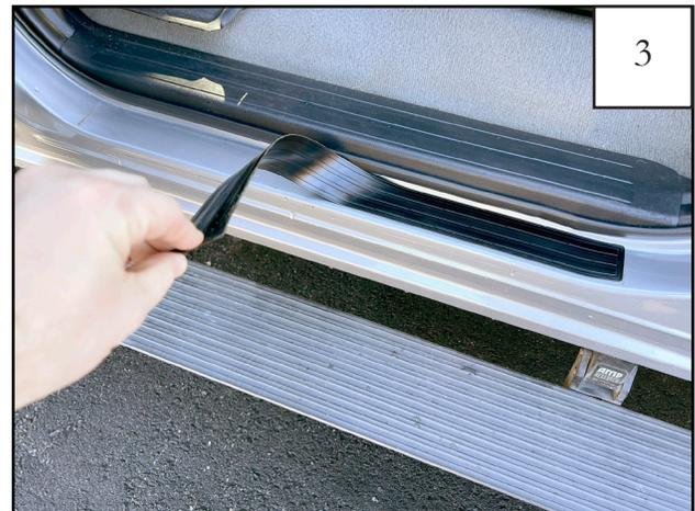
Carefully remove the factory installed stick-on plate.
