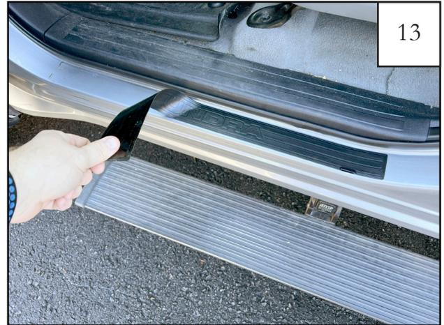
Carefully remove the factory installed stick-on plate.
