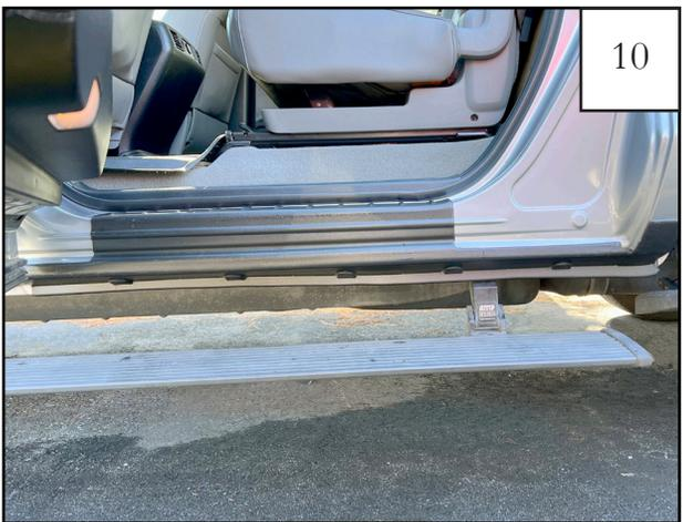
Once all tape liners are peeled, press down on entire length of part applying strong force to taped areas.
