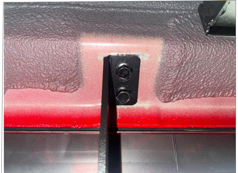
5. Next, adjust the step assembly up/down and front/back to level out the step rail with body panel and then tighten step to brackets at 20 ft. /lbs
