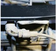
Spring installed on top of OE center block.
