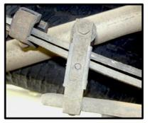
Remove roller from rear rebound bracket. Do not remove bracket.
