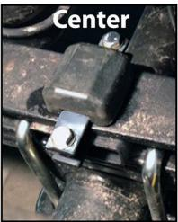
Mounting kit installed with bumpstop
