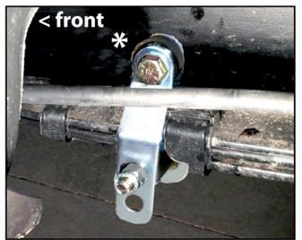
\*eye bolt threads inward roller bolt threads outward
