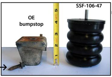
Thread the OE self-tapping screw into the threaded bolt hole on the frame several times to allow for installation of the SSF-106. Install by threading jounce into the existing hole.
