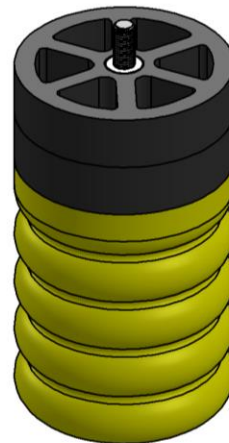
BOTH SPACERS INSTALLED WITH 90MM BOLT
