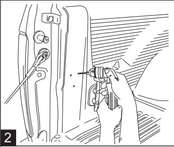
Cut out supplied template and tape to the D-pillar as shown. Using a center punch, mark holes as specified by the template.
