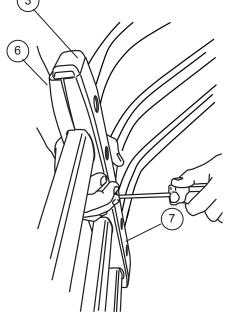
NOTE: Do not over tighten as this may strip out. Fastener will reach a noticeable stopping point.
