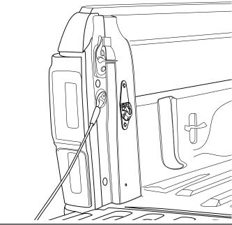
Tighten fasteners. Make sure pivot opening in bracket opens towards the rear of the vehicle.
