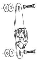
Passenger side, Bracket and hardware orientation
