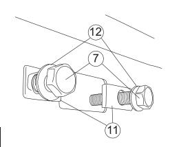
Mount idler assembly and motor assembly. Note: Filing of sheet metal edge may be required if the sheet metal holes are misaligned.
