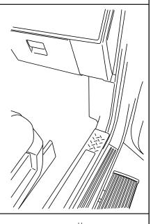
Remove tape from 3/4" hole in floor panel above front linkage on passenger side and insert grommet. Thread all four trigger wires through grommet up into the cabin of vehicle. Seal grommet with silicone sealer.
