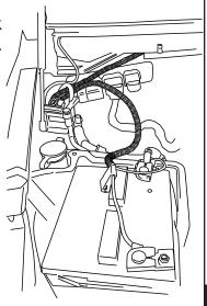
Route longer wire harness leg across firewall through plastic cowling to driver side.
