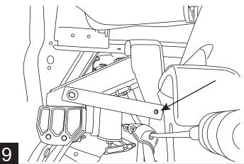
Install rearward support bracket (#6) using supplied M8 Hardware(#8) Bolts and (#9) Nuts. Torque to 16Ft-Lbs.
