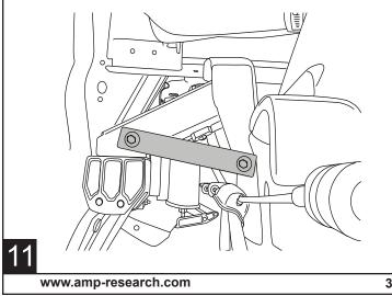
Install forward support bracket (#5) using supplied M8 hardware (#8) bolts and (#9) nuts. Torque bolts to 16Ft-Lbs.
