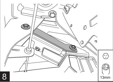
Remove bracket and pre drill hole using a 1/8" drill bit then drill to 3/8".
