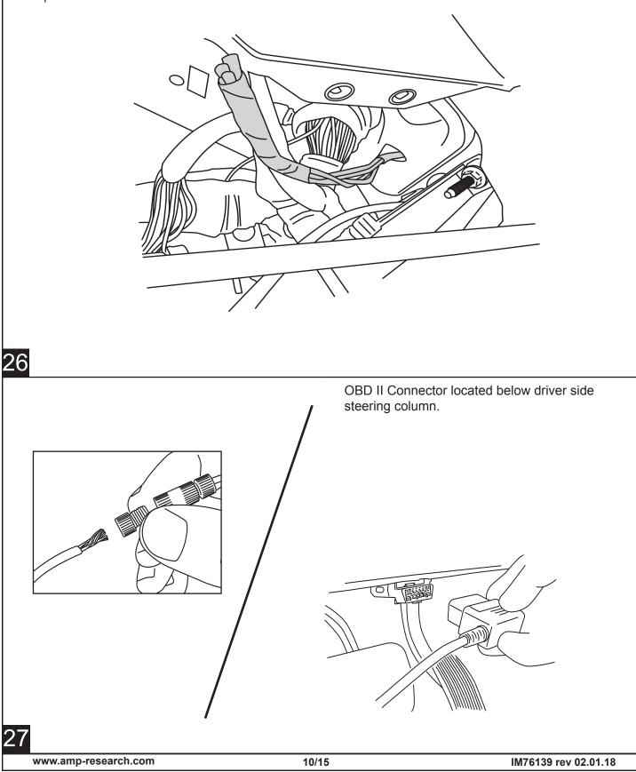
**OBD II install:** Use Supplied Posi Twist connectors to attach the Plug and Play Module to the Harness. Attach matching colors on the harness to the wires on the module. Plug in module to OBD II port on the vehicle. Secure harness with supplied tie wraps.
