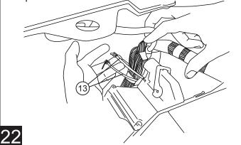
Remove fuse from Power Step Wire Harness.
