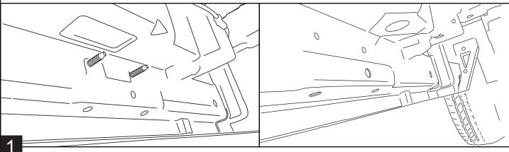
To attach the **Rear Motor Linkage** to the rear factory-step mount location, when no studs/threaded inserts are present, the three holes need to be drilled to the proper size **17/32**" to install three Rivet nuts (#7) using the supplied Rivet nut tool (#16). Next, install the **Rear Motor Linkage** (#3) using three Conical bolts (#6),
