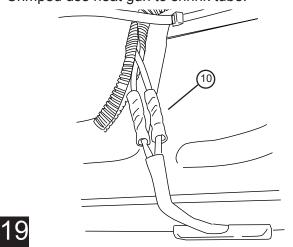
Close and wrap with conduit and electrical tape. Secure all loose wires with cable ties, with lamp wires pulled upward to avoid any wire snagging.
