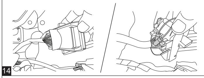
Once the trigger wire has been connected to the OBDII module (#18), remove the OBDII port from the vehicle by depressing the two plastic tabs on the sides and push the port back out of the bracket. Now connect the OBDII module to the OBDII port.
