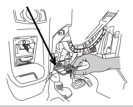
**OBD II install:** Use Supplied Posi-Lock™ connectors to attach the Plug and Play Module to the Harness. Attach matching colors on the harness to the wires on the module. Plug in module to OBD II port on the vehicle. Secure harness with supplied tie wraps. *Note: If the OBD II pass thru harness (76404-01A) was purchased see install sheet supplied in packaging. The pass through harness allows for an open port for other accessories. See below for a brief description.*
