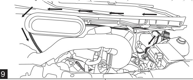
Route wire harness along the upper side of the floor/ rocker structure directly towards the front linkage. Secure with zip ties (#11). Keep away from exhaust components.
