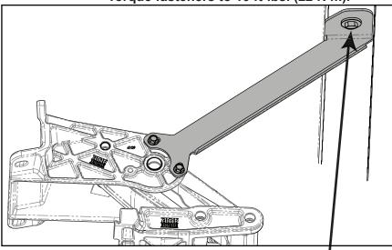
To attach the **Rear Bracket (#21)** to the rear linkage, start by using the Thread Cutting bolt (#23), to cut threads in the blank insert in the frame rail. Use a 9/16" socket and rachet, go slow and stay straight. Then install the bracket on the non-motor side of linkage loosely with two bolts(#22), install the upper Bolt (#23) and Washer (#24), loosely and tighten the bottom two bolts fully. Now, tighten the top.
