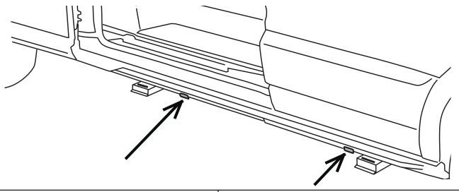
Affix lamps to rocker panel surface. Make sure the lamp is affixed to a clean. flat surface. The outside the rocker face is the ideal location affix the lamp just at its edge. If already equipped with a step, the rear door rocker will be different but the light shall
