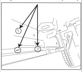
Torque fasteners to 10 ft-lbs. (22 N m).
