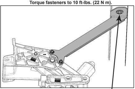
To attach the **Rear Bracket (#20)** to the rear linkage, start by using the Thread Cutter bolt (#22), to cut threads in the blank insert in the frame rail. Use a 9/16" socket and rachet go slow and stay straight. Then install the bracket on the non-motor side of linkage loosely with two bolts(#21), install the upper Bolt (#22) and Washer (#23), loosely and tighten the bottom two bolts fully. Now, tighten the top.
