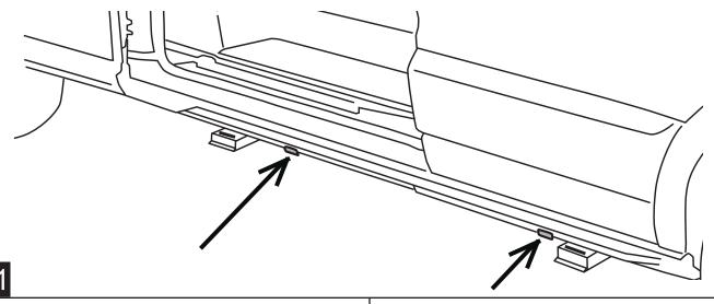
Affix lamps to rocker panel surface. Make sure the lamp is affixed to a clean, flat surface. The outside the rocker face is the ideal location affix the lamp just at its edge. If already equipped with a step, the rear door rocker will be different but the light shall be placed in the position shown in the previous step.
