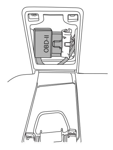
The Clip-In Pass-Though Harness is available if it is desired to have an open OBDII port in the stock location.
