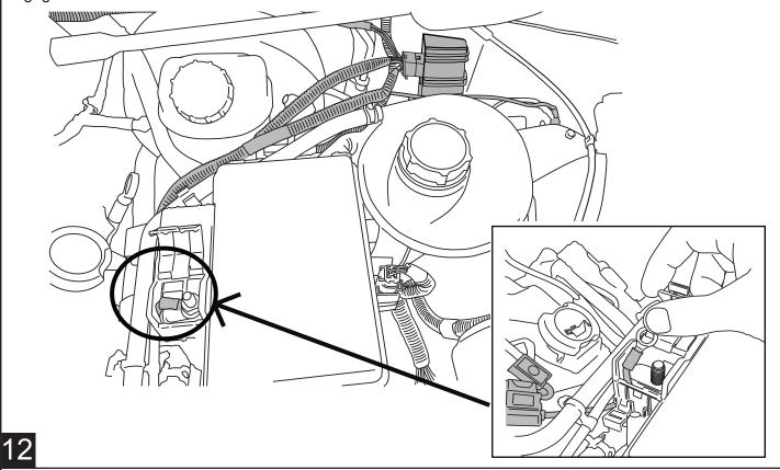
Route long end of wire harness above engine and down through passenger side wheel well. Zip tie the harness to cowling clips on fire wall. Route the short end down through driver side wheel well. Keep away from exhaust and steering components. Secure with zip ties (#20).
