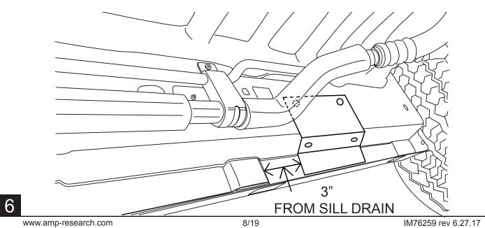
Next, install the Driver Bracket to the front face of the Front Driver Linkage and the vertical plate on the frame as shown blelow, there is an existing hole present. Use bolt (#21), bolt (#6), and Nut (#8). If the rear AC lines are present the bracket will go between them.
