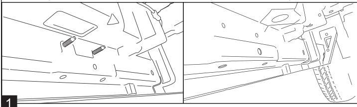
To attach the **Rear Motor Linkage** to the rear factory-step mount location, when no studs/threaded inserts are present, the three holes need to be drilled to the proper size **17/32**" to install three Rivnuts (#7) using the supplied Rivnut tool (#15). Next, install the **Rear Motor Linkage** (#3) using three Conical bolts (#6), start by installing the upper bolt loosely, then install and tighten the bottom two bolts fully. Now, tighten the top.
