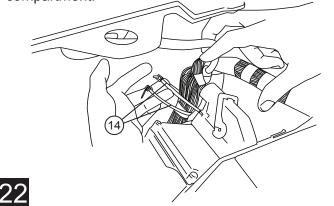
Remove fuse from Power Step Wire Harness.
