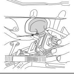
Tape leading end of wires together and push through rubber boot to cabin side of the firewall. Silicon lubricant may be used for ease of passage. The trigger wires will come out just above and to the left of the brake pedal.
