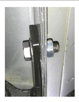
**Step. 6:** After finial positioning, completely tighten all (x4)  $\frac{1}{2}$ "-20 x  $\frac{3}{4}$ " in the pinch weld attachment.
