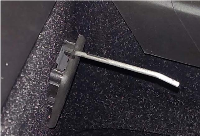
1. Use the included tool to remove the USB receptacle.
