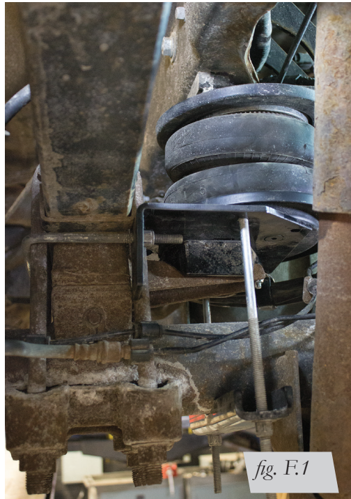
Back, driver's (left) side rear view of the kit installed.
