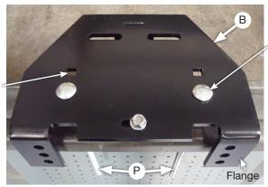
For models with sway bars, right (passenger side) only, use these holes for installing Carriage Bolts (B).
