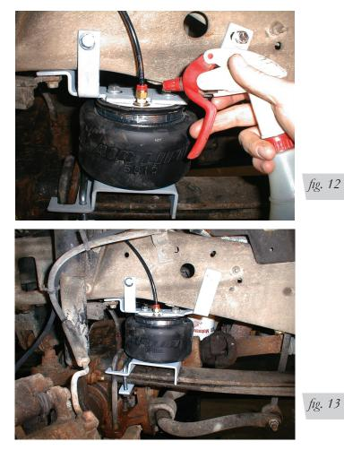
3. After the test, deflate the springs to the minimum pressure required to restore the system to normal ride height. Do not deflate to lower than 5 PSI.
