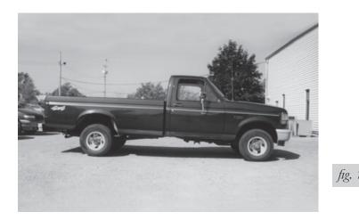
2. Measure the distance between the center of the hub and the bottom edge of the wheel well (see Fig. 2). This is the Normal Ride Height. Enter the measurement below:
