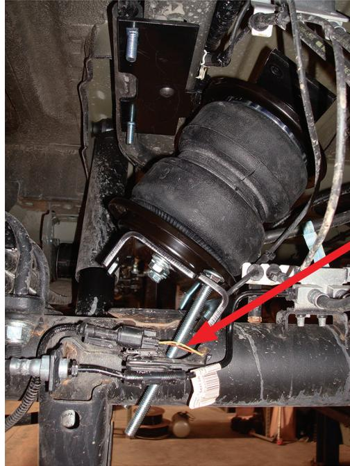
Left side shown: set one of the assemblies into position making sure that the carriage bolt goes in between the brake/ABS lines and the axle as shown.
