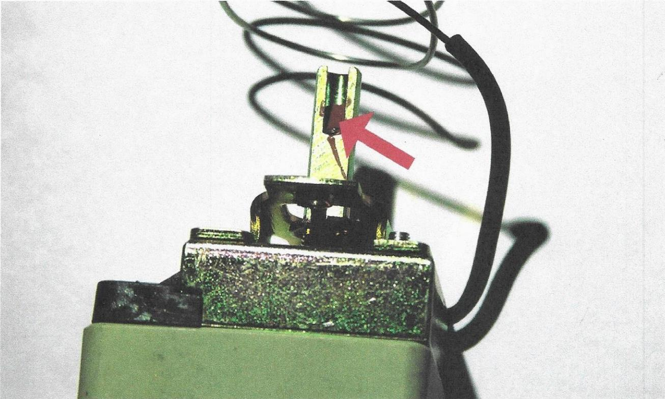
This Red rubber sealant must be removed to access the calibration screw. The image below shows the area after the sealant has been removed.
