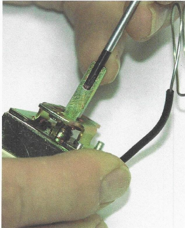
**NOTE:** Hold the outer shaft firmly while making adjustments to the calibration screw.
