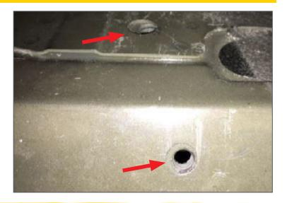
Step 2. Next, start x3 (#3) M8X30mm Hex Cap bolts in the upper mounts only and leave loose. NOTE: **Make sure you only engage enough threads so the bolt can easily slide through the upper mount attachment point.**
