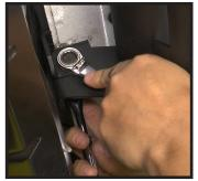
STEP 15 (Passenger Side): Snug hardware for the first and second bracket. Tighten the bolt going up throught the pinch weld first to pull the board into place. Then tightening both side bolts.
