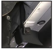
STEP 13 (Passenger Side): Use 13mm bolt to align 2 piece bracket to the board, insert at the sideand hand tighten. Apply to both first and second bracket.
