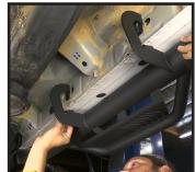
STEP 12 (Passenger Side): Carefully place passenger side step into place. Use bolt, washer and begin hand tightening both upper mountings and pinch weld mounting to the rear two brackets Best to have a assistant to lift and hold board in place.
