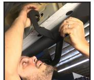
**STEP 16** (Passenger Side): **Avoid using power or air tools.** Tighten pinch weld mounts first then upper bolts. Tighten all hardware to 20ft lbs torque to secure the board to the truck.
