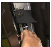
**STEP 14** (Passenger Side): Insert bolt and washer going up through board, truck pinch weld and through the 2 piece bracket.
