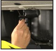
**STEP 11** (Passenger Side): Take bracket and feed between the body and the DEF tank from the back of the tank. You'll be able to fit and hand tighten bolt through the bracket to the body.
