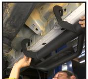
STEP 12 (Passenger Side): Carefully place passenger side step into place. Use bolt, washer and begin hand tightening both upper mountings and pinch weld mounting to the rear two brackets Best to have a assistant to lift and hold board in place.
