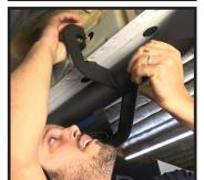
**STEP 16** (Passenger Side): **Avoid using power or air tools.** Tighten pinch weld mounts first then upper bolts. Tighten all hardware to 20ft lbs torque to secure the board to the truck.
