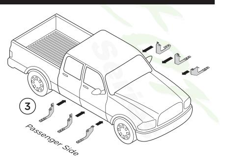
**4.** Install the Front Passenger Side Bracket closest to the front wheel. Align with existing factory holes in the rocker panel as shown (4a), Secure the Front Passenger Side Bracket using two (2) M10 x 30mm Hex Bolts, two (2) M10 Lock Washers and two (2) M10 Flat Washers (4b).
