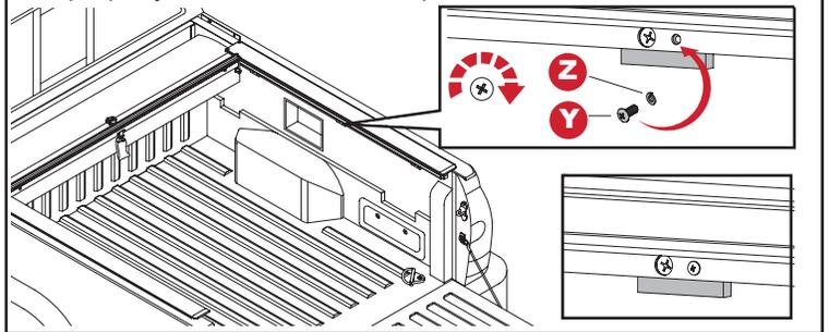
**9C FOR 05-15 TACOMA INSTALL** - Lower the tailgate and place the tailgate extrusion (R) assembly onto tailgate.
