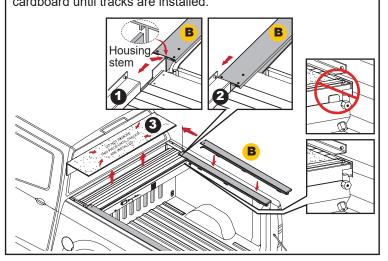
**10** Secure tracks (B) to housing stem (1) on driver and passenger side using cargo nut (H) and #10-24 screw (O) using a Phillips screwdriver (2).
