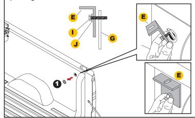
**9** (1) Loosely attach the CM track bracket (E) to the pre-in stalled track clamp with 1/4" flat washer (N) and 1/4" socket cap screw (M). (2) Loosely attach CM bed clamps (f) to the pre-installed track clamps using 5/16" socket cap screw (K) and 5/16" lock washer (L) on driver and passenger side.
