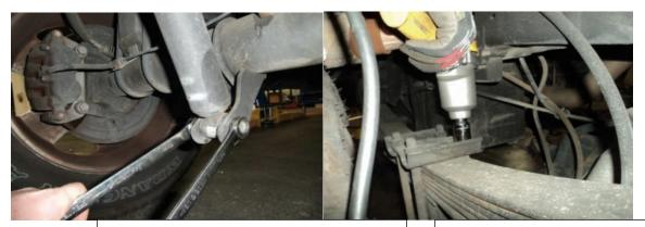
Remove the lower shock mount hardware.
