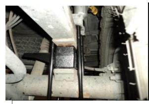
Make sure block pins are aligned properly in axle and leaf pack. Align u-bolts and tighten, perform the following steps on the opposite side. Lower vehicle to ground and torque ubolts to factory specs. Double check all work and test drive vehicle. Have your vehicle aligned and enjoy.
