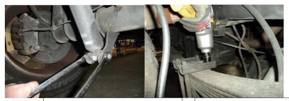
Remove the lower shock mount hardware.
