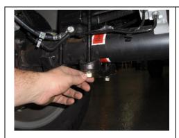
Attach lower mounting plate with provided hardware.
