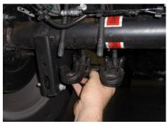
Remove u-bolt nuts and lower plate.
