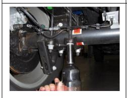
Loosen and remove factory u-bolt hardware.
